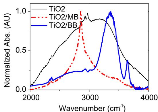
**Fig. 3** The normalized FTIR absorption spectrum of the  $\text{TiO}_2$  ( $\text{TiO}_2$ ), Mondo-grass berry extract coated on  $\text{TiO}_2$  ( $\text{TiO}_2/\text{MB}$ ) and Blackberry extract coated on  $\text{TiO}_2$  ( $\text{TiO}_2/\text{BB}$ )
