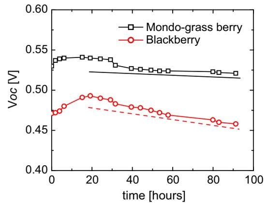
Fig. 6 The stability comparison between Mondo-grass and blackberry soaked DSSCs,  $V_{oc}$  of each cell is monitored by refilling the electrolyte each time
