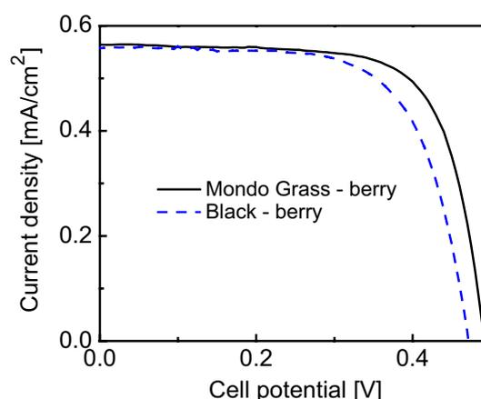
**Fig. 4** IV Characteristics of the solar cells loaded with Mondo-grass berry and Blackberry dyes, the samples were measured using KETHLEY 2400 source meter
