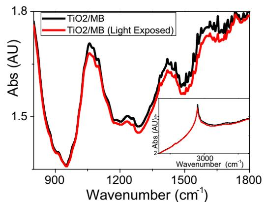
Fig. 7 The IR absorption spectra of Mondo berry extract just after coating the on  $TiO_2$  and after light soaking (~8 h)
