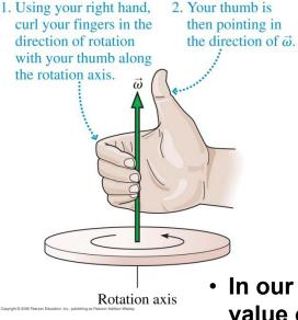
USING VECTORS TO DESCRIBE ROTATIONAL KINEMATICS AND DYNAMICS:
