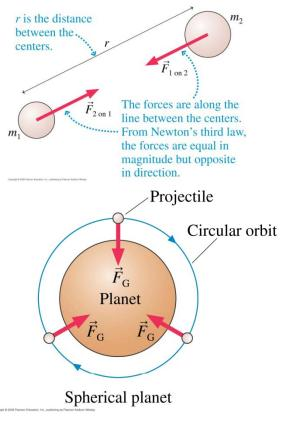
$$F_{G} = G \frac{m_{1}m_{2}}{r^{2}} = m_{satellite} \left( G \frac{m_{E}}{r_{orbit}^{2}} \right) = m_{satellite} \left( \frac{v_{satellite}^{2}}{r_{orbit}} \right)$$
