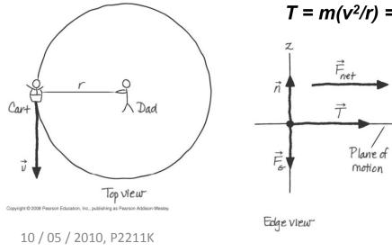
$T = m(v^2/r) = (25 \text{ kg}) (2.5 \text{ m/s})^2 / 2.0 \text{ m} = 78.13 \text{ N}$
