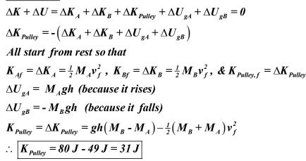
b. Calculate the rotational inertia of the pulley. (10 pts)
