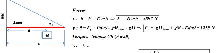
$$\left(\frac{L}{2}\right)gM_{beam} + dgM = LTsin\theta \implies T = \frac{\left(\frac{L}{2}\right)gM_{beam} + dgM}{Lsin\theta} = 4500 N$$
