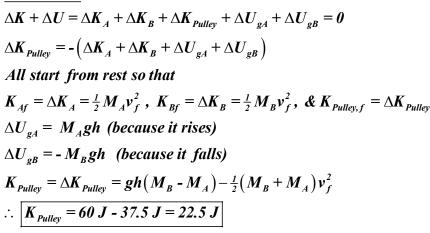
b. Calculate the rotational inertia of the pulley. (10 pts)
