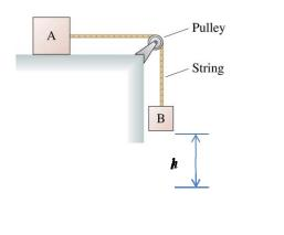
$\frac{Basic \ idea :}{\Delta K + \Delta U = \Delta K_A + \Delta K_B + \Delta U_g = 0}$ (a) start,  $K_{Ai} = K_{Bi} = 0$ (a) end,  $K_{Af} = \frac{1}{2}M_A v^2$  &  $K_{Bf} = \frac{1}{2}M_B v^2$ (a) start,  $U_g = M_B gh$  (choose  $y_i$  as h, which makes  $y_f = 0$ )
