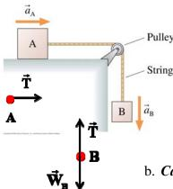
$$\begin{aligned} m_{A}a &= T \\ m_{B}a &= W_{B} - T = m_{B}g - T = m_{B}g - m_{A}a \\ a &= \frac{m_{B}g}{m_{A} + m_{B}} = \frac{80N}{20kg} = 4 \text{ m/s}^{2} \end{aligned}$$
