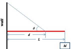
*a.* Calculate the horizontal and vertical components of the force on the beam from the connection to the wall.  $F_x = 22733 N; F_y = -625 N$
