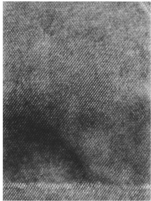
Fig. 3. Cross sectional HREM image of a GaP/Si(100) interface prepared by CBE using TEG and TBP as source materials.
