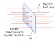
The magnetic flux is proportional to the number of field lines that pass through a surface.
