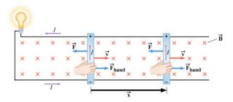
In order to keep the rod moving at constant velocity, the force the hand exerts on the rod must balance the magnetic force on the current:
