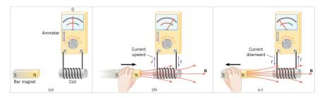
The current in the coil is called the *induced current* because it is brought about by a changing magnetic field.
