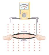
In each example, both an emf and a current are induced because the coil is part of a complete circuit. If the circuit were open, there would be no induced current, but there would be an induced emf.
