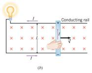
The separated charges on the ends of the conductor give rise to an induced emf, called a *motional emf.*
