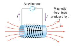
The effect in which a changing current in a circuit induces and emf in the same circuit is referred to as *self induction*.
