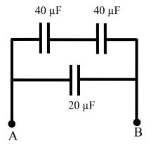
7. What is the equivalent capacitance between points A and B?
